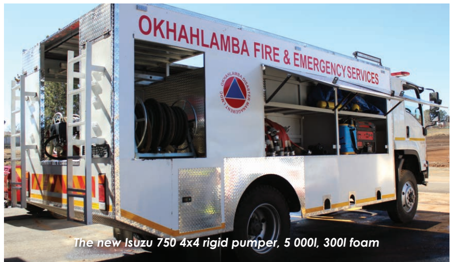
The new Isuzu 750 4x4 rigid pumper, 5 000l, 300l foam
